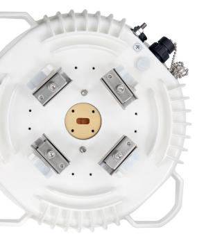
CFIP-106/108 is primarily designed for IP networks and provides Fast Ethernet interface with capacities from 8 Mbps up to 100 Mbps full duplex Fast Ethernet. In addition to that, CFIP-106/108 has a 4xE1/T1 port for legacy equipment connectivity and for use in hybrid TDM/IP networks.
